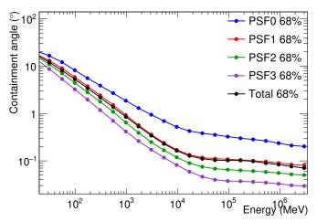
**Figure 1.** Containment angle (68%) of the *Fermi*-LAT PSF as a function of energy, averaged over off-axis angle. The black line is the average over all data, whereas the colored lines illustrate the difference between the four categories of events ranked by PSF quality from worst (PSF0) to best (PSF3).
