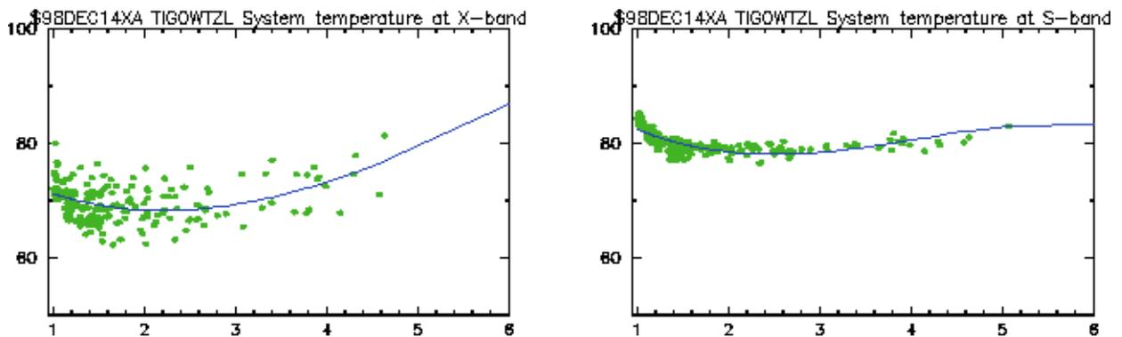
Fig. 3: System temperature in X- and S-band versus number of air masses.
