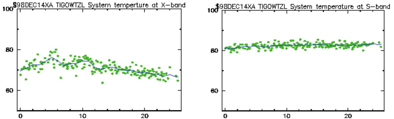
Fig. 2: System temperature in X- and S-band versus time in hours during EUROPE-46.
