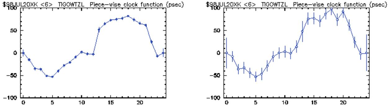
Fig. 4: Clock behavior of TIGOWTZL relative to WETTZELL in phase delay and group delay solution after removal of linear trend. Argument is time in hours.
