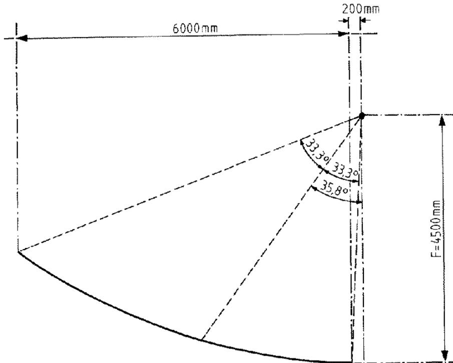
Fig. 1: Optical scheme of the antenna
